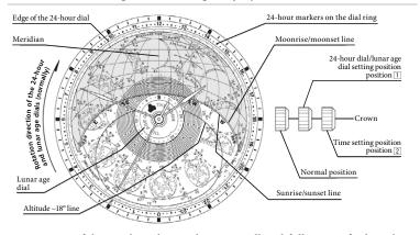
Distortion of the southern hemisphere is small and full range of celestial sphere where the Sun and Moon pass at 35° N is displayed. (Northern limit of the celestial sphere displaying part overlapping 24-hour dial: Declination +29.25°)
