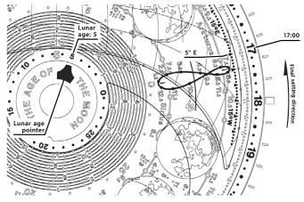
Align the first left  $\triangle$  (5° to the 15°E direction) from the center  $\triangle$  (marker nearest of the analemma) with 17:00 of the 24-hour markers on the dial ring.
