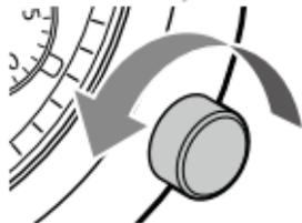
When the screw lock is released, the crown extends to the normal position.
