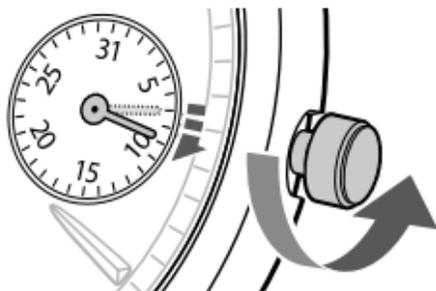
Rotate the crown to the left (counterclockwise) to set the date. (The date does not change when you rotate the crown to the right (clockwise).)
