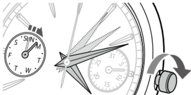
Rotate the crown to the right (clockwise) to set the day. (The day hand moves when the hour hand is indicating between 0 a.m. and 5 a.m.)
