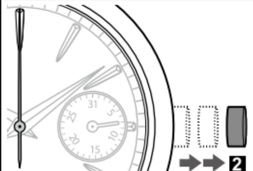
With the second hand in the 0-second position, pull the crown out two 'steps' to position 2.
