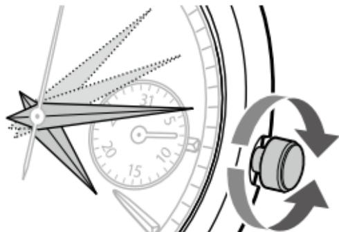
Rotate the crown to set the time, paying attention to a.m. and p.m.
