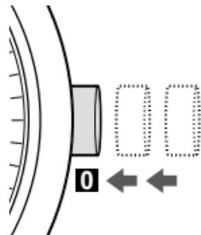
Return the crown to the normal position (**0**) in sync with a reliable time source.
